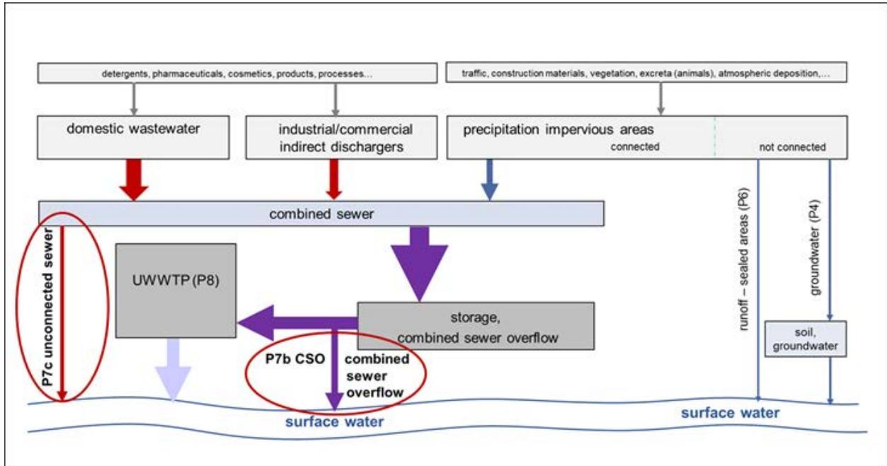
Figure 6.2: Schematic overview of emissions to surface waters via combined sewer systems including combined sewer overflows (CSO) and unconnected combined wastewater sewer
